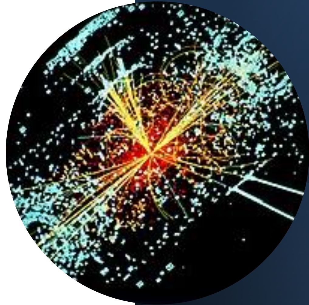
Simulated Large Hadron Collider CMS particle detector data depicting a Higgs boson produced by colliding protons decaying into hadron jets and electrons
